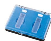
Glass Cuvette (2ea/box) Item no. 3-574-02 Volume: 3.5 ml Optical path distance (mm): 10
